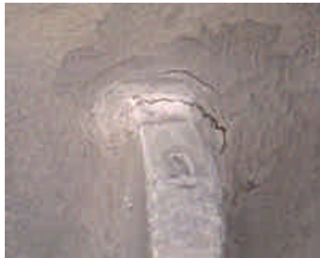
Figure 3.1 b A weld after 1.5 mm of grinding.
