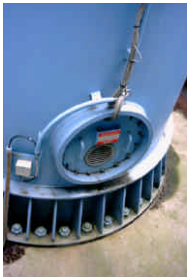
Figure 2.2 h The modified base details and details of the inspection door. The cables above the inspection door are a part of the data collecting system.
