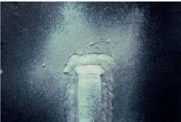
Figure 15. Fatigue crack detected by magnetic-particle testing at the toe between two weld passes around a vertical stiffener at the base of the chimney in Figures 13 and 14
